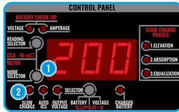
If your battery does not fit the options, use the nearest smallest value, and in case there is more than one battery in parallel in the system, add the amperage of all and select the capacity that most closely closes to that of the seat.
