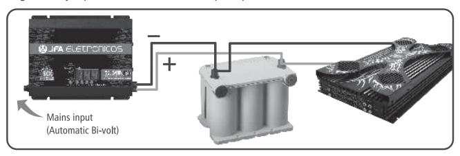
You can use as many sources 36A, 50A, 60A, 70A, 100A, 120A, 150A and 200A as needed to feed the sound, having as a reference that each one maintains about 1800, 2500, 3000, 3500, 4400, 6000, 7000 and 10000 Wrms of sound playing respectively, it is important to note that for this the operating mode must be the same for all sources that are in parallel (ex.: All in 14.4V mode or all in Auto SCI).
