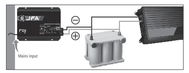
You can use as many Sources 60A, 80A, 120A and 200A as necessary to feed the sound, having as reference that each one keeps about 3,000, 4,000, 6,000, and 10,000 Wrms of sound playing respectively, it is important to note that when operating in In parallel, the sources must operate in the same MODES as follows:
